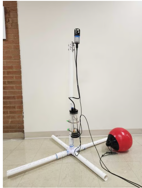
Fig. 2. Custom-built PVC frame used to mount static beacons in the test environment. The modular and lightweight design allows for rapid deployment and recovery of SeaTrac X150 USBL acoustic modems. Although USBL devices were used for signal collection, our RSS-based localization method does not rely on their full positioning capabilities.
